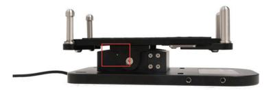
When this LED is green, the Foot Control is operational. When the LED is off, the Foot Control isn't powered. When this LED flashes red, it indicates additional faults, to these in Error codes on page 44. Count the flashes and contact mo-vis for more information: contact@mo-vis.com.
