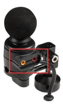
has 2 switches that can be linked to the separate interface: (1) on/off power wheelchair - (2) mode of the power wheelchair.
