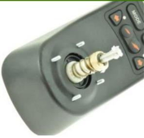
A close-up photograph of the joystick assembly. A brass-colored metal axle is inserted into a black plastic housing. The axle has a sliding bush and a spring. The housing has several screws around the joystick opening. To the right, there are some buttons and a 'STOP' label. |
