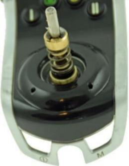
A close-up view of the joystick axle assembly. A white grease applicator is shown applying grease to the top of the joystick axle. The axle is surrounded by a sliding bush and a spring. The joystick housing is black, and the base of the joystick is visible, showing the letters 'G' and 'M'.                 |
