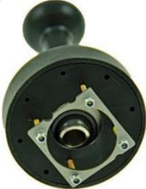
A top-down view of the joystick assembly. A black circular reinforcement plate is being lifted away from the central joystick mechanism. The plate has four screws and washers around its perimeter. The joystick's internal components, including a central bush and spring, are visible through the center hole. |
